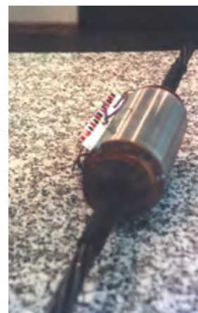
Figure 3: Design and assembly of the sensor around of the cable.
